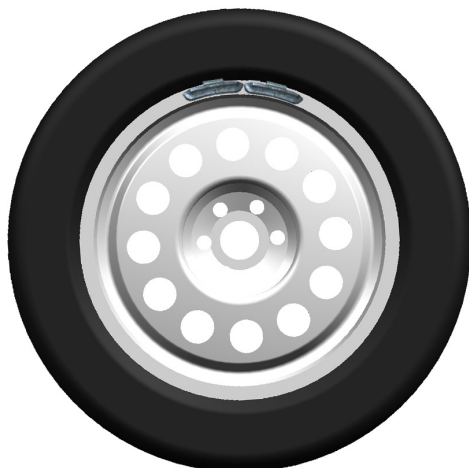
TWO SMALLER WEIGHTS (50g) (1.76 oz) FITTED MANUALLY
