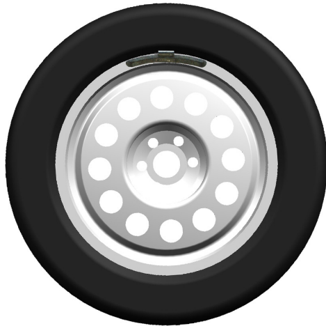
100 g (3.52 oz) WEIGHT TO BE FITTED TO CORRECT UNBALANCE
