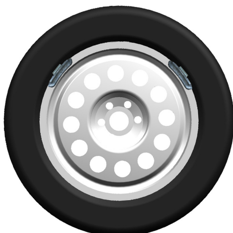
TWO SMALLER WEIGHTS (55g) (1.94 oz) USING SPLIT PROCEDURE
