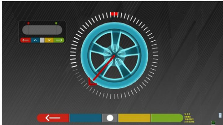
At this point, it is necessary to rotate the wheel until the position indicator is aligned with the second point, positioned at 180° with respect to the first position and thus coinciding with the starting point.
