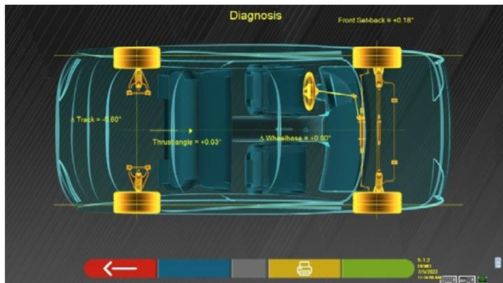
This measurement is made during vehicle alignment (Para. 7.9). Differences in wheelbase and track width and front axle setback are displayed on this page.
