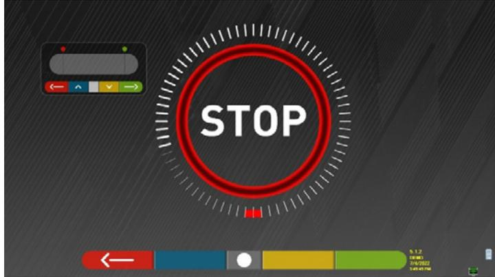
The word "STOP" will be displayed for about three seconds, the time it takes for the program to acquire the measurements.
