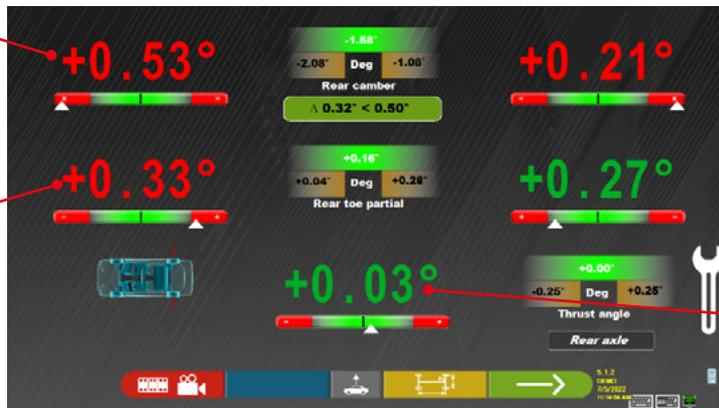
Thrust angle measurements.
