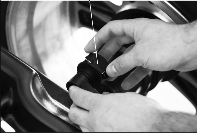
Fig. 47 Fit the adhesive weight in the pliers of the gauge rod
