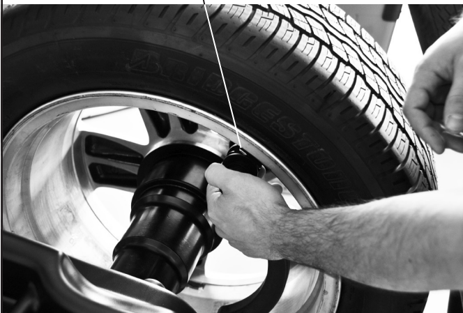
Fit weight on the position where pliers touches the wheel Fig. 48
